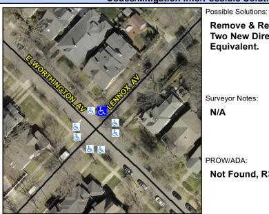
**LENNOX AV** Street 1 Name StopSign Stop Condition-Street 1 Street 2 Name N/A Stop Condition-Street 2 N/A **Remove & Replace Curb Ramp With** Two New Directional Ramps or Equivalent.
