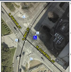
W STONEWALL ST Street 1 Name Stop Condition-Street 2 Signal Street 2 Name N/A Stop Condition-Street 1 N/A Possible Solutions: Remove & Replace Entire Ramp. Surveyor Notes: N/A PROW/ADA: Not Found, R304.2.2, R304.5.3
