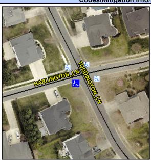
Street 1 Name Stop Condition-Street 2 Street 2 Name Stop Condition-Street 1 **TODDINGTON LN** None HARLINGTON LN StopSign Possible Solutions: Remove & Replace Curb Ramp With **Two New Directional Ramps or** Equivalent. Surveyor Notes: N/A PROW/ADA: Not Found, R304.5.1, R304.5.3
