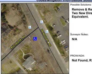
Street 1 Name Stop Condition-Street 2 Street 2 Name Stop Condition-Street 1 **RANDOLPH RD** None **RUTLEDGE AV** StopSign Remove & Replace Curb Ramp With **Two New Directional Ramps or** Equivalent.
