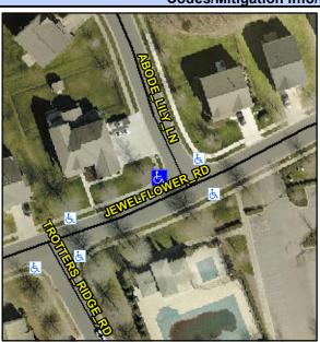
Street 1 Name Stop Condition-Street 2 Street 2 Name Stop Condition-Street 1 JEWELFLOWER RD None **ABODE LILY LN** StopSign Possible Solutions: Remove & Replace Curb Ramp With **Two New Directional Ramps or** Equivalent. Surveyor Notes: N/A PROW/ADA: Not Found, R304.5.1, R304.2.2
