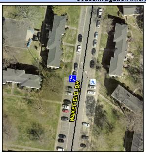
**WAKEFIELD DR** Street 1 Name Stop Condition-Street 1 None Street 2 Name N/A Stop Condition-Street 2 N/A Possible Solutions: Remove & Replace Curb Ramp With Two New Directional Ramps or Equivalent. Surveyor Notes: **CROSSES PARKING SPACES** PROW/ADA: R304.5.3, R304.2.2-Perp, R304.3.2-Para, R305.2
