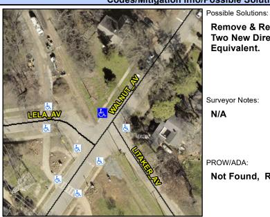
**WALNUT AV** Street 1 Name Stop Condition-Street 1 StopSign Street 2 Name N/A Stop Condition-Street 2 N/A Remove & Replace Curb Ramp With Two New Directional Ramps or Equivalent.
