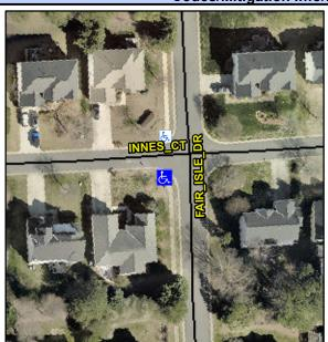
FAIR ISLE DR Street 1 Name Stop Condition-Street 2 **INNES CT** Street 2 Name Stop Condition-Street 1 StopSign Possible Solutions: Remove & Replace Curb Ramp With Two New Directional Ramps or Equivalent. Surveyor Notes: N/A PROW/ADA: R304.5.3
