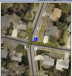
WILD DOVE LN Street 1 Name Stop Condition-Street 2 Street 2 Name **CHARTER HILLS RD** Stop Condition-Street 1 StopSign Possible Solutions: **Remove & Replace Curb Ramp With Two New Directional Ramps or** Equivalent. Surveyor Notes: N/A PROW/ADA: Not Found, R304.5.1, R304.2.2, R304.5.3
