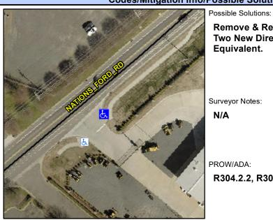
NATIONS FORD RD Street 1 Name Stop Condition-Street 2 Street 2 Name **ENTRANCE** Stop Condition-Street 1 StopSign **Remove & Replace Curb Ramp With Two New Directional Ramps or** Equivalent.
