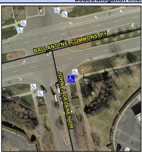
JOHN J DELANEY DR Street 1 Name Stop Condition-Street 1 StopSign Street 2 Name N/A Stop Condition-Street 2 N/A Possible Solutions: Remove & Replace Curb Ramp With **Two New Directional Ramps or** Equivalent.
