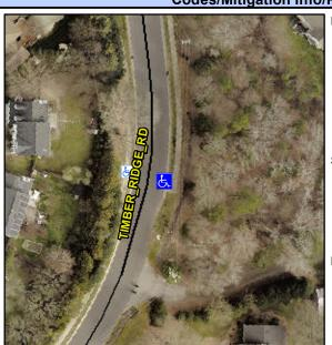
**TIMBER RIDGE RD** Street 1 Name Stop Condition-Street 2 None Street 2 Name N/A Stop Condition-Street 1 N/A Possible Solutions: Remove & Replace Entire Ramp. Surveyor Notes: N/A PROW/ADA: Not Found, R304.2.2, R304.5.3
