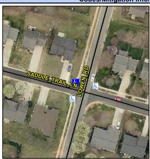
SADDLE TRAIL LN Street 1 Name Stop Condition-Street 2 StopSign **LOWEN RD** Street 2 Name Stop Condition-Street 1 None Possible Solutions: Remove & Replace Curb Ramp With Two New Directional Ramps or Equivalent. Surveyor Notes: N/A PROW/ADA: Not Found, R304.5.1, R304.5.3
