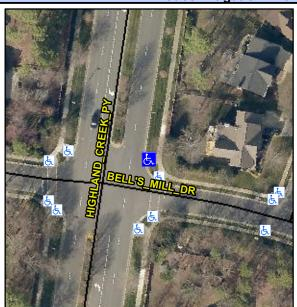
**BELL'S MILL DR** Street 1 Name Stop Condition-Street 2 None Street 2 Name N/A Stop Condition-Street 1 N/A Possible Solutions: Remove & Replace Entire Ramp. Surveyor Notes: N/A PROW/ADA: R304.5.1, R304.2.2, R304.5.3
