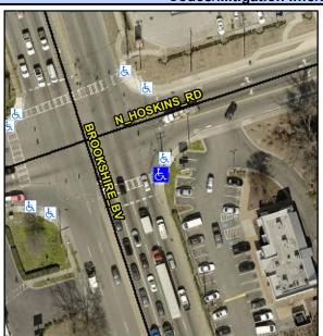
**BROOKSHIRE BV** Street 1 Name Stop Condition-Street 1 Signal Street 2 Name N/A Stop Condition-Street 2 N/A Possible Solutions: Remove & Replace Entire Ramp. Surveyor Notes: RT RP < 5% PROW/ADA: R304.3.2, R304.5.3
