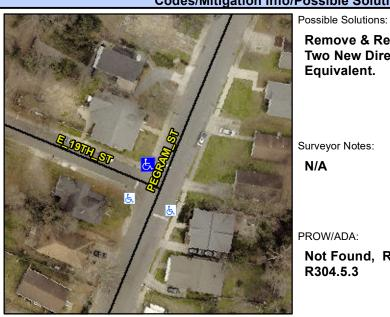
E 19TH ST Street 1 Name Stop Condition-Street 2 StopSign Street 2 Name **PEGRAM ST** Stop Condition-Street 1 StopSign Remove & Replace Curb Ramp With Two New Directional Ramps or Equivalent.
