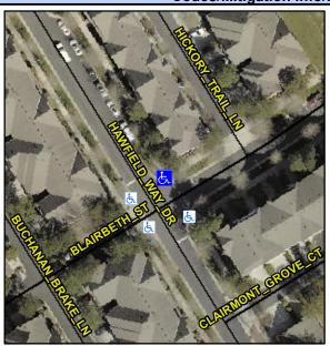
Street 1 Name Stop Condition-Street 2 Street 2 Name Stop Condition-Street 1 HAWFIELD WAY DR StopSign **BLAIRBETH ST** StopSign Possible Solutions: Remove & Replace Curb Ramp With **Two New Directional Ramps or** Equivalent. Surveyor Notes: N/A PROW/ADA: Not Found, R304.5.3
