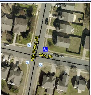
**FOX POINT DR** Street 1 Name Stop Condition-Street 2 StopSign Street 2 Name OAK DR Stop Condition-Street 1 None Possible Solutions: Remove & Replace Curb Ramp With **Two New Directional Ramps or** Equivalent. Surveyor Notes: N/A PROW/ADA: Not Found, R304.5.1, R304.2.2
