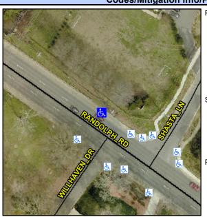
RANDOLPH RD Street 1 Name Stop Condition-Street 2 None Street 2 Name N/A Stop Condition-Street 1 N/A Possible Solutions: Remove & Replace Entire Ramp. Surveyor Notes: N/A PROW/ADA: Not Found, R304.2.1, R304.2.2-Perp, R304.3.2-Para, R304.5.3
