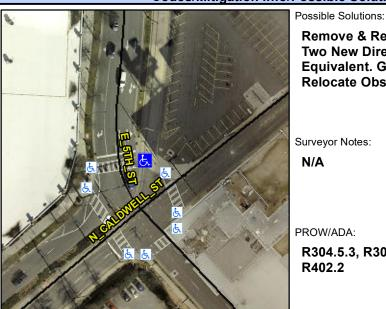
E 5TH ST Street 1 Name Stop Condition-Street 1 Signal Street 2 Name N/A Stop Condition-Street 2 N/A Remove & Replace Curb Ramp With Two New Directional Ramps or Equivalent. Grind Gutter Lip. Relocate Obstruction.
