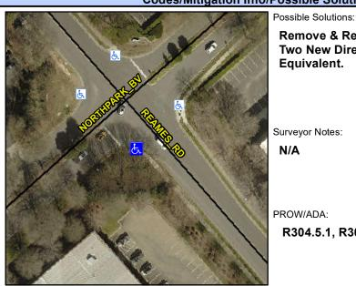
**REAMES RD** Street 1 Name Stop Condition-Street 2 None Street 2 Name **NORTHPARK BV** Stop Condition-Street 1 StopSign **Remove & Replace Curb Ramp With Two New Directional Ramps or** Equivalent.
