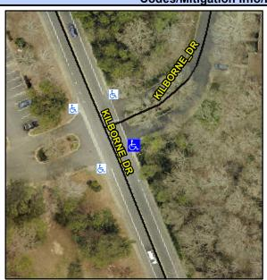
Street 1 Name Stop Condition-Street 2 Street 2 Name Stop Condition-Street 1 KILBORNE DR None **KILBORNE DR** None Possible Solutions: Remove & Replace Curb Ramp With Two New Directional Ramps or Equivalent. Surveyor Notes: N/A PROW/ADA: R304.5.1, R304.2.2, R304.5.3
