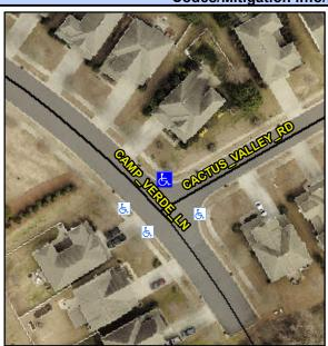
Street 1 Name **CAMP VERDE LN** Stop Condition-Street 2 **CACTUS VALLEY RD** Street 2 Name Stop Condition-Street 1 StopSign Possible Solutions: Remove & Replace Curb Ramp With Two New Directional Ramps or Equivalent. Surveyor Notes: N/A
