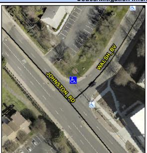
Street 1 Name Stop Condition-Street 2 Street 2 Name Stop Condition-Street 1 JOHNSTON RD None **WALSH BV**  Remove & Replace Curb Ramp With **Two New Directional Ramps or** Equivalent.
