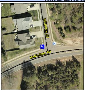
Street 1 Name Stop Condition-Street 1 Street 2 Name Stop Condition-Street 2 Possible Solutions: Remove & Replace Curb Ramp With Two New Directional Ramps or Equivalent. Surveyor Notes: RT RP < 5%
