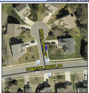
WHITE BARN CT Street 1 Name Stop Condition-Street 1 None Street 2 Name N/A Stop Condition-Street 2 N/A Possible Solutions: Remove & Replace Curb Ramp With **Two New Directional Ramps or** Equivalent. Surveyor Notes: N/A PROW/ADA: Not Found, R304.2.1, R305
