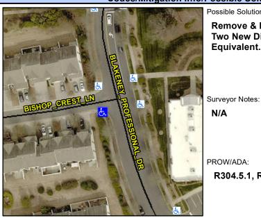
**BLAKENEY PROFESSIONAL DR** Street 1 Name Stop Condition-Street 1 None Street 2 Name **BISHOP CREST LN** Stop Condition-Street 2 StopSign Possible Solutions: **Remove & Replace Curb Ramp With** Two New Directional Ramps or Equivalent.
