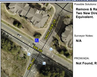
Street 1 Name IBM DR Stop Condition-Street 2 Signal **NEAL RD** Street 2 Name Stop Condition-Street 1 Signal Remove & Replace Curb Ramp With Two New Directional Ramps or Equivalent.
