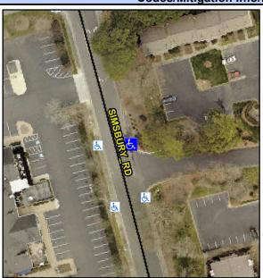
SIMSBURY RD Street 1 Name Stop Condition-Street 2 None **ENTRANCE** Street 2 Name Stop Condition-Street 1 None Possible Solutions: Remove & Replace Curb Ramp With Two New Directional Ramps or Equivalent. Surveyor Notes: N/A PROW/ADA: R304.2.2, R304.5.3
