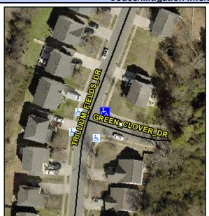
Street 1 Name TRILLIUM FIELDS DR Stop Condition-Street 2 **GREEN CLOVER DR** Street 2 Name Stop Condition-Street 1 StopSign Possible Solutions: Remove & Replace Curb Ramp With Two New Directional Ramps or Equivalent. Surveyor Notes: N/A PROW/ADA: R304.5.1
