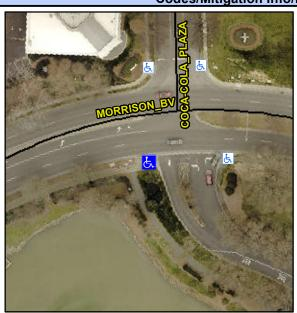
Street 1 Name **COCA-COLA PLAZA** Stop Condition-Street 2 None Street 2 Name **MORRISON BV** Stop Condition-Street 1 None Possible Solutions: Remove & Replace Curb Ramp With **Two New Directional Ramps or** Equivalent. Surveyor Notes: N/A PROW/ADA: Not Found, R304.2.2
