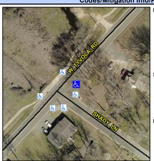
Street 1 Name None W TYVOLA RD Stop Condition-Street 1 Street 2 Name N/A Stop Condition-Street 2 N/A Possible Solutions: Remove & Replace Entire Ramp. Surveyor Notes: RT RP < 5% PROW/ADA: Not Found, R304.5.1, R304.3.2, R304.5.3
