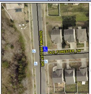
Street 1 Name Stop Condition-Street 2 Street 2 Name Stop Condition-Street 1 **SONOMA VALLEY DR** None **OLD FORESTER LN** StopSign Possible Solutions: **Remove & Replace Curb Ramp With Two New Directional Ramps or** Equivalent. Surveyor Notes: N/A PROW/ADA: Not Found, R304.5.1
