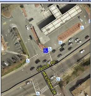
**WESTPARK DR** Street 1 Name Signal Stop Condition-Street 2 **TYVOLA RD** Street 2 Name Stop Condition-Street 1 Signal Possible Solutions: Remove & Replace Curb Ramp With Two New Directional Ramps or Equivalent. Surveyor Notes: N/A PROW/ADA: Not Found, R304.5.1
