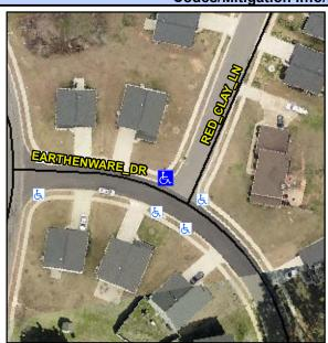
**EARTHENWARE DR** Street 1 Name Stop Condition-Street 2 **RED CLAY LN** Street 2 Name Stop Condition-Street 1 StopSign Remove & Replace Curb Ramp With Two New Directional Ramps or Equivalent.
