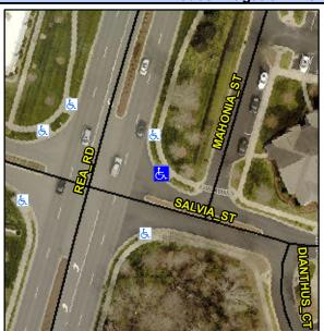
**REA RD** Street 1 Name Stop Condition-Street 2 YieldSign Street 2 Name **BLAKENEY PARK DR** Stop Condition-Street 1 StopSign Possible Solutions: **Remove & Replace Curb Ramp With Two New Directional Ramps or** Equivalent. Surveyor Notes: N/A PROW/ADA: Not Found, R304.5.1, R304.2.2, R304.5.3
