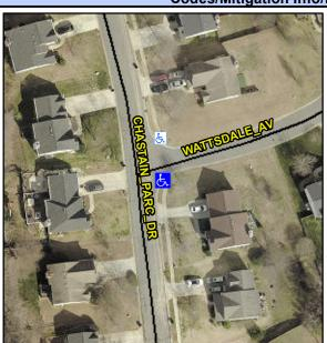
**WATTSDALE AV** Street 1 Name Stop Condition-Street 1 StopSign Street 2 Name N/A Stop Condition-Street 2 N/A Possible Solutions: Remove & Replace Curb Ramp With **Two New Directional Ramps or** Equivalent. Surveyor Notes: N/A PROW/ADA: Not Found, R304.5.1, R304.5.3
