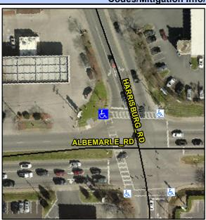
ALBEMARLE RD Street 1 Name Stop Condition-Street 2 Signal Street 2 Name HARRISBURG RD Stop Condition-Street 1 Signal Possible Solutions: Remove & Replace Curb Ramp With **Two New Directional Ramps or** Equivalent. Surveyor Notes: N/A PROW/ADA: Not Found, R304.2.2
