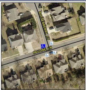
**PAULINE LN** Street 1 Name Stop Condition-Street 2 None **BOYSENBERRY CT** Street 2 Name Stop Condition-Street 1 StopSign Possible Solutions: Remove & Replace Curb Ramp With **Two New Directional Ramps or** Equivalent. Surveyor Notes: N/A PROW/ADA: Not Found, R304.5.3
