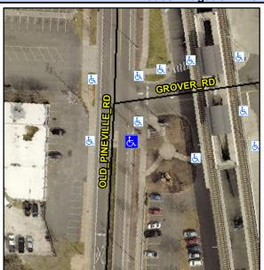
**OLD PINEVILLE RD** Street 1 Name Stop Condition-Street 2 None Street 2 Name N/A Stop Condition-Street 1 N/A Possible Solutions: Remove & Replace Entire Ramp. Remove & Replace Gutter. Surveyor Notes: N/A PROW/ADA: Not Found, R304.5.3
