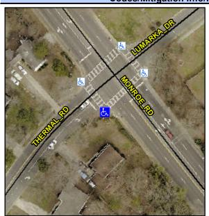
MONROE RD Street 1 Name Stop Condition-Street 2 Signal **LUMARKA DR** Street 2 Name Stop Condition-Street 1 Signal Possible Solutions: Compliance Description N/A Remove & Replace Curb Ramp With Two New Directional Ramps or Yes Equivalent. N/A N/A N/A N/A Surveyor Notes: N/A N/A N/A N/A N/A N/A PROW/ADA: N/A Not Found, R304.2.2 N/A N/A N/A
