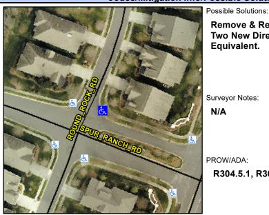
Street 1 Name Stop Condition-Street 2 Street 2 Name Stop Condition-Street 1 **ROUND ROCK RD** StopSign **SPUR RANCH RD** None Remove & Replace Curb Ramp With Two New Directional Ramps or Equivalent.
