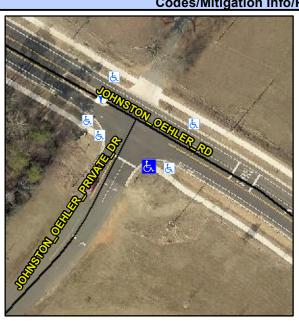
JOHNSTON OEHLER PRIVATE DR Street 1 Name Stop Condition-Street 1 StopSign N/A Street 2 Name Stop Condition-Street 2 N/A Possible Solutions: Remove & Replace Curb Ramp With Two New Directional Ramps or Equivalent. Surveyor Notes: N/A PROW/ADA: R304.5.3
