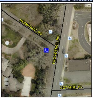
Street 1 Name Stop Condition-Street 2 Street 2 Name Stop Condition-Street 1 PROVIDENCE RD None **HERMITAGE RD** StopSign Possible Solutions: **Remove & Replace Curb Ramp With** Two New Directional Ramps or Equivalent. Surveyor Notes: N/A PROW/ADA: Not Found, R304.5.1, R304.2.2, R304.5.3
