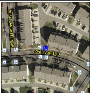
KING LOUIS CT Street 1 Name Stop Condition-Street 2 None N/A Street 2 Name Stop Condition-Street 1 None Possible Solutions: Remove & Replace Curb Ramp With Two New Directional Ramps or Equivalent. Surveyor Notes: N/A PROW/ADA: R304.5.1, R304.2.2, R304.5.3
