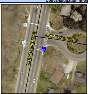
Street 1 Name Stop Condition-Street 1 Street 2 Name Stop Condition-Street 2 W SUGAR CREEK RD Signal **HIDDEN VALLEY RD** Signal Possible Solutions: Remove & Replace Curb Ramp With Two New Directional Ramps or Equivalent. Surveyor Notes: LT RP < 5% PROW/ADA: R304.5.1, R304.3.2
