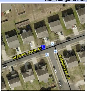
**REDDING GLEN AV** Street 1 Name Stop Condition-Street 1 None Street 2 Name N/A Stop Condition-Street 2 N/A Possible Solutions: **Remove & Replace Curb Ramp With Two New Directional Ramps or** Equivalent. Surveyor Notes: N/A PROW/ADA: Not Found, R304.2.2-Perp, R304.3.2-Para, R305
