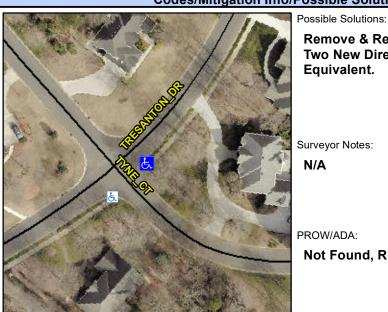
Remove & Replace Curb Ramp With Two New Directional Ramps or Equivalent.
