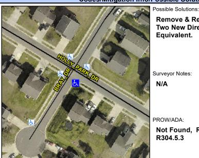
**HOLLY PARK DR** Street 1 Name Stop Condition-Street 2 None **BRAY DR** Street 2 Name Stop Condition-Street 1 StopSign Remove & Replace Curb Ramp With Two New Directional Ramps or Equivalent.
