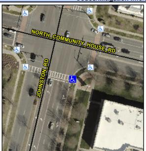
JOHNSTON RD Street 1 Name Stop Condition-Street 2 Signal Street 2 Name N/A Stop Condition-Street 1 N/A Possible Solutions: Remove & Replace Entire Ramp. Surveyor Notes: N/A PROW/ADA: R304.5.1, R304.5.3
